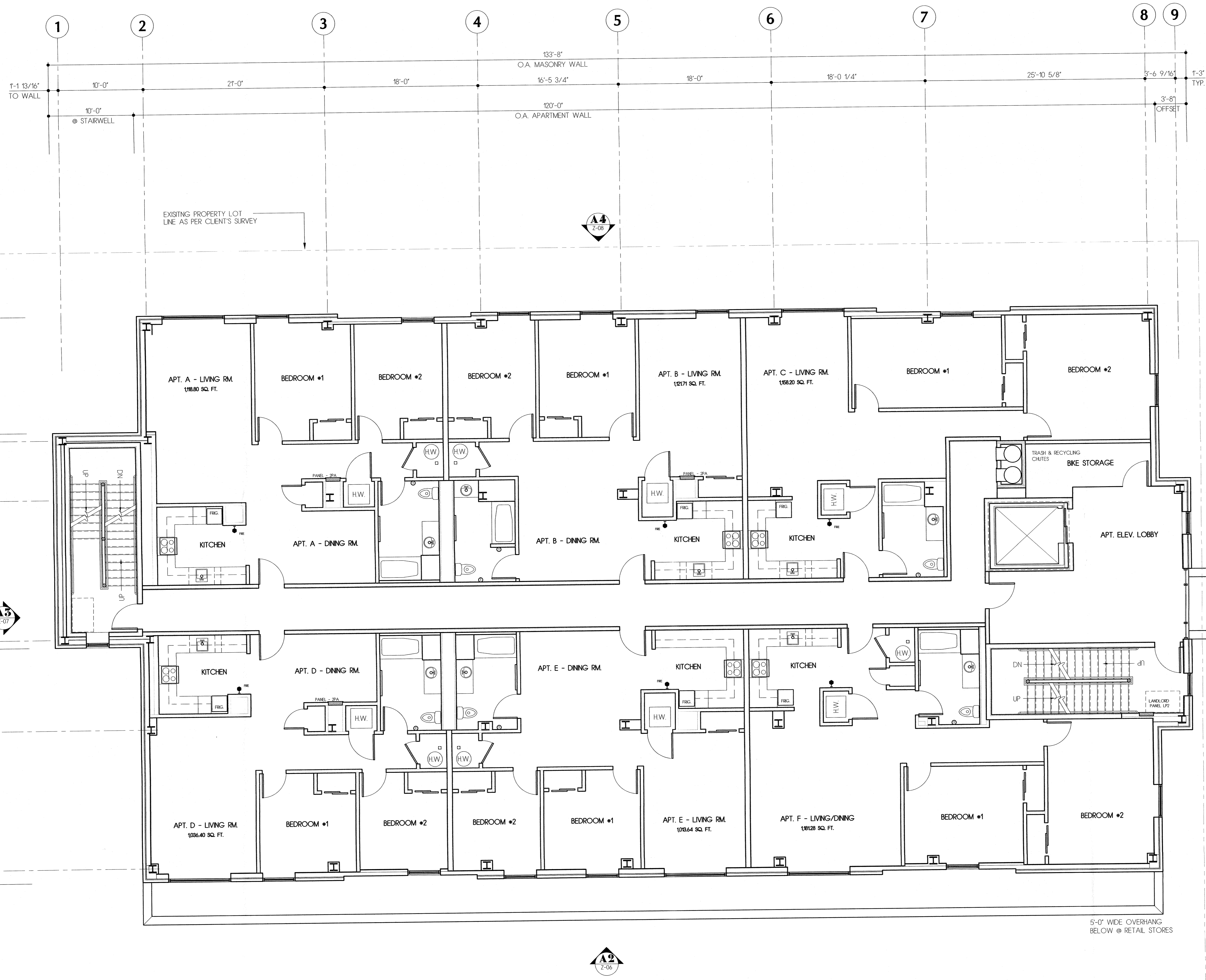
2 SECOND & THIRD FLOOR APARTMENT PLAN DIAGRAM SCALE: 3/16" = 1'-0" APT. FLOOR AREA = 8,362.11 GROSS SQ. FT.
